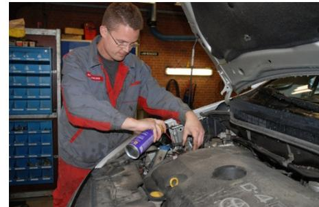
Electrical Connections are treated with ‘Prolan’ to prevent corrosion and moisture penetration.
